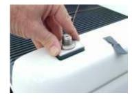
When tape shim is just the right size, the mount will slip into place if you moisten the tape slightly and push it down into place.
