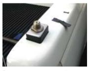
Put more tape around the top of the mount than you think necessary. Check for spacing. Then, remove tape a little at a time as necessary to achieve a tight fit.
