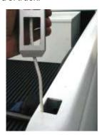
Route the coax down the stake pocket and through the washers and anchor bolt hole.
